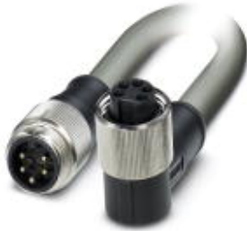
Bus system cable, DeviceNet, 5-position, PVC, Gray RAL 7001, Plug straight 7/8"-16UNF, on Socket angled 7/8"-16UNF, Cable length: 0.5 m
