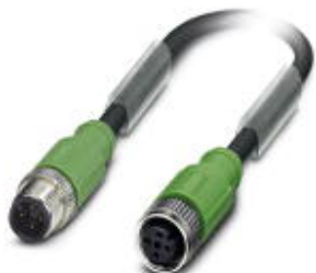
Sensor/actuator cable, 4-position, PUR/PVC, black-gray RAL 7021, shielded, Plug straight M12, A-coded, on Socket straight M12, A-coded, cable length: 0.6 m
